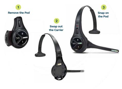
The G5 Headset is the first headset with a modular design. Being modular, the parts are removable for easy repairs and service. Simply remove the battery, remove the pod, & you have an empty carrier!
